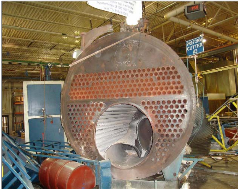
Tube Damage After Dry Fired Explosion
