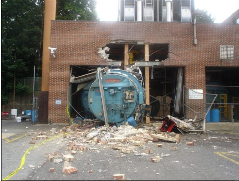
Fire Tube Boiler Exploded And Came Through The Wall Of A Hospital
