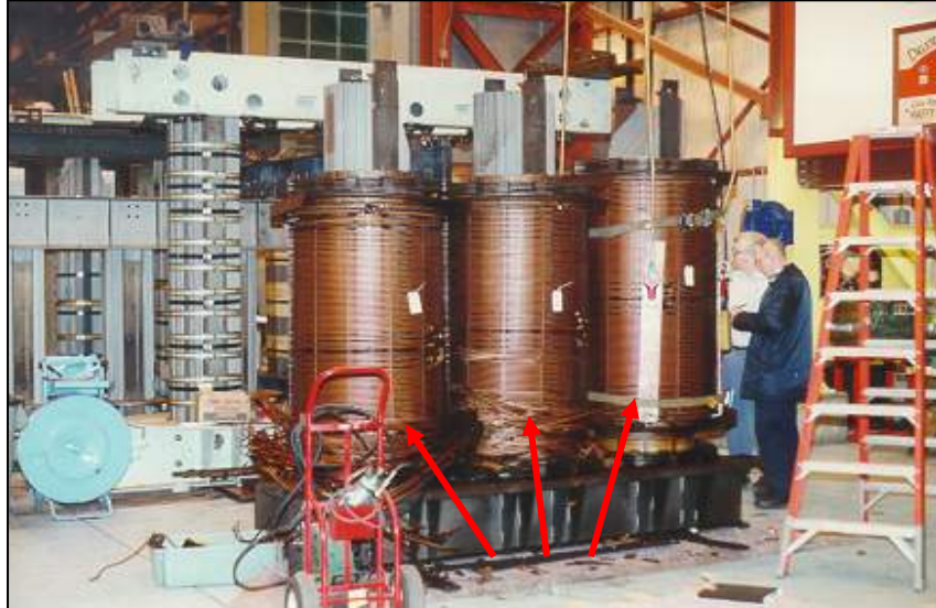
Transformer With Damaged Windings
