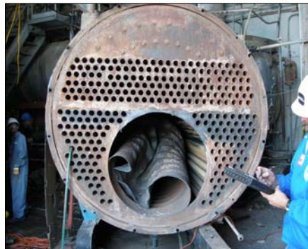
Fire Box Collapse – Caused By A Low Water Condition
